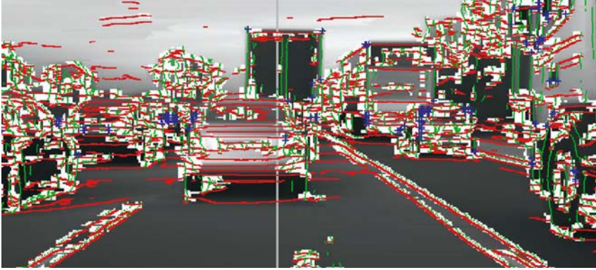
Figure 5.41. “Imagined” feature set extracted with the unified blob-edge-corner method UBM: Linearly shaded blobs (gray areas), horizontally (green) and vertically extracted edges (red), corners (blue crosses) and nonhomogeneous regions (white).
