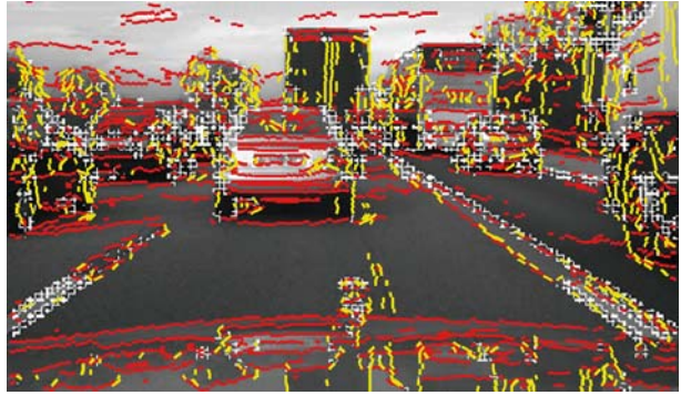
Figure 5.30. Edges from extreme values in gradient components in row (yellow) and column search (red, parameters m, n : m_c, n_c = 33.21 ), \text{IntGradMin} = 0.016 ; white regions are bi-directionally nonplanar features.
