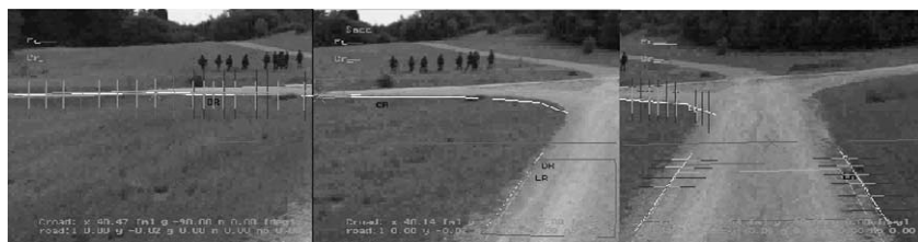
Figure 14.13. Tele-images during saccadic vision while approaching a crossroad; the center image during a saccade is not evaluated (missing indicated search paths)
