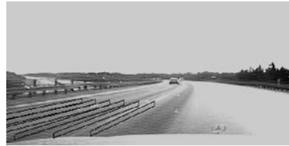
Figure 11.30. Definition of regions for detecting passing vehicles: In the road direction, extended vertical rectangles of predefined height are positioned (virtually) side by side in the near range along the neighboring lane just above the ground
