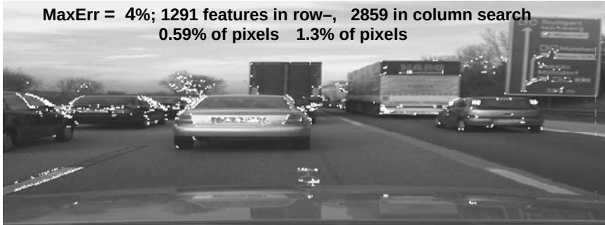
Figure 5.22. Nonplanarity features in central rectangle of an original video-field (cell size m_c = 1 , n_c = 1 , mel size 1 \times 1 , finest possible resolution, \text{MaxErr} = 4\% )
