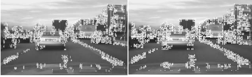
Figure 5.27. Nonplanar features for parameter set ErrMax = 2.5%, mask elements m = n = 2 and cell size n_c = m_c = 2 (i.e., first pyramid level, left; after processing compressed 2:1 in rows for better comparison). Changing m_c to 4 (right) yields about the same number of features : \sim 2500 .
